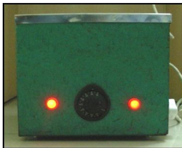
Figure 5B: Custom-made apparatus for 48-hour load relaxation tests- lateral view.
