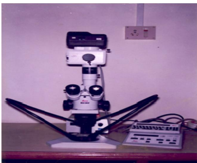
Fig 3: Stereomicroscope (Leica Wild M3Z)
